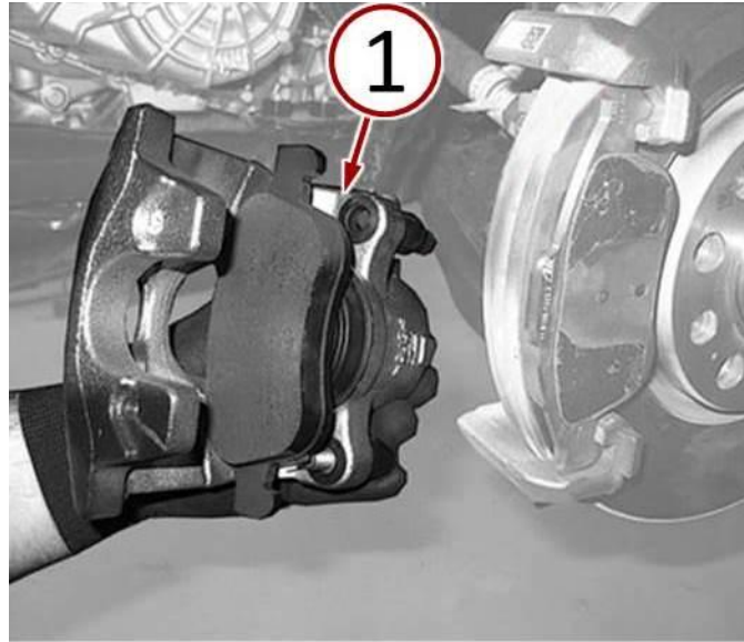
Fig. 2 Remove And Support Brake Caliper
