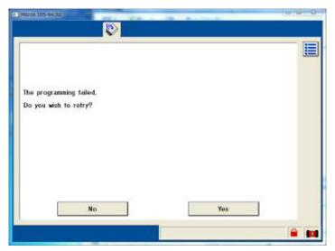
b. If the screen shows "The programming failed." without Yes/No buttons, the ABS module has to be replaced with new one.
