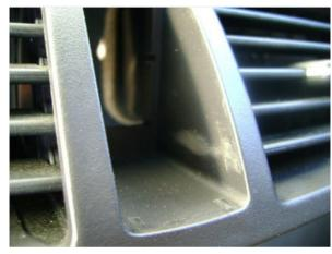
To check for this, just pull out the switch and look for signs of rubbing in the panel opening. If you see any, you probably just need to replace the panel and **not** the switch.
