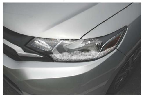
Condensation is a normal occurrence and should dissipate on its own.
