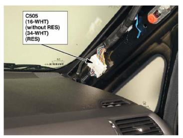
To fix this problem, check the connector and reset it if needed. If the connection is good, continue with normal troubleshooting.
