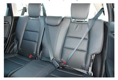
Don't unbolt the lower anchor plates to uncross the seat belts. Such a change in the belts' configuration, could affect their level of protection.
