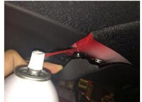
3. Apply dry lube to the lower stopper bracket area.
