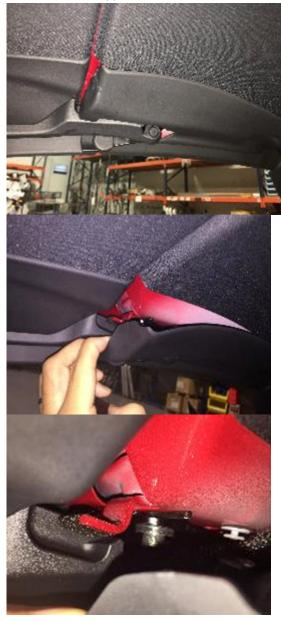
2. Apply dry lube to the upper / back area of the stopper bracket.
