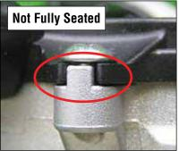
15) Connect wiper motor wiring connector.
