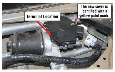
12) Press down the wiper motor bottom cover gently and evenly over the terminal location to insure that the terminal is properly seated in the terminal socket.
