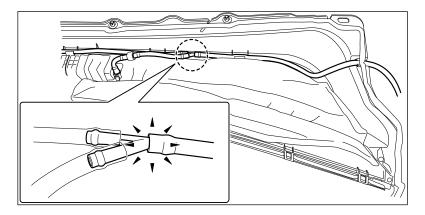
6) CAREFULLY disconnect wiring harness connector from wiper motor.
