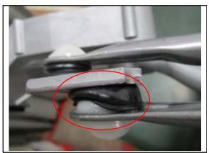
2. Pull back the rubber seal to prevent damage when performing the following steps.
