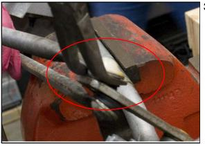
3. Use bent needle nose pliers to separate the wiper link rod from the wiper link assembly.
