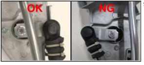
Install the wiper link plate to the wiper motor shaft.
