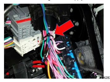
20. Return the spliced wires into the UBEC splash shield between the connectors, routing them so they will not be crushed during the UBEC re-installation. Using a tie strap, secure the spliced wires near the existing tie strap on the engine harness connector.
