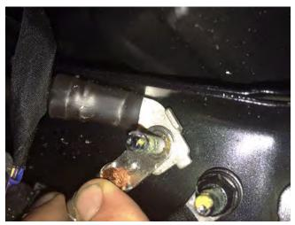
15.4 Install the ground cable from the battery to the G100 ground stud, then install the modified terminal with di-electric grease to the stud.
