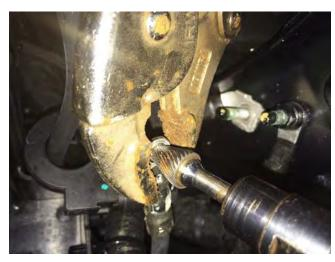
15.1 Using a cone shaped rotary file, or equivalent, open up the inside diameter of the eyelet by approximately 0.4mm.
