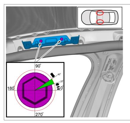
Warning! Loosen the screw between 20-40 degrees.
