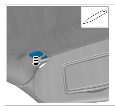
Remove the marked part. On both sides.
