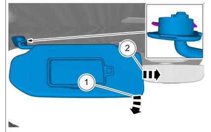
Remove the part carefully Fold marked part to one side. On both sides.
