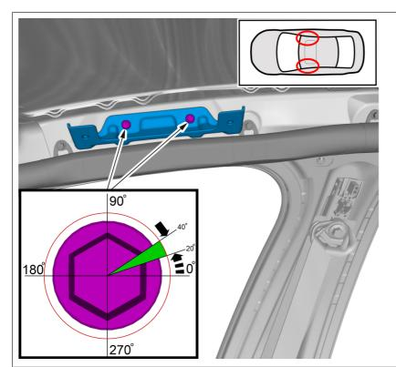
Warning! Loosen the screw between 20-40 degrees.
