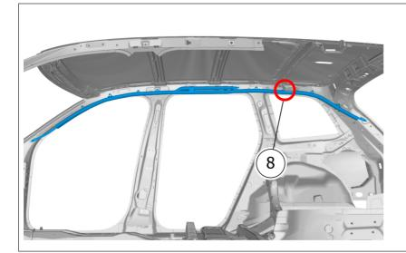
Bolt in position 8 is located behind rear load net retainer bracket. On both sides.
