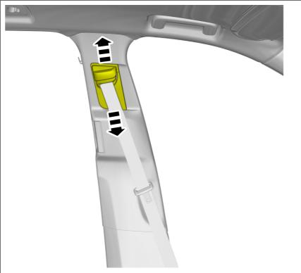
Check for correct operation. On both sides.
