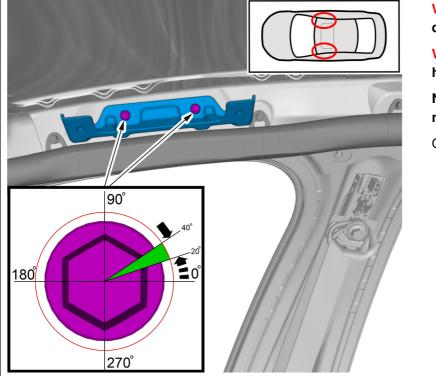
Warning! Loosen the screw between 20-40 degrees.
