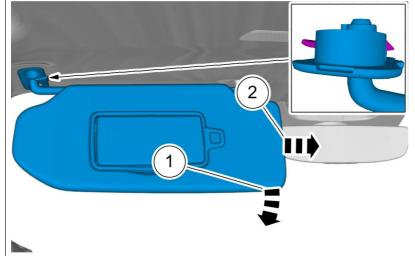
Remove the part carefully Fold marked part to one side. On both sides.
