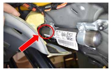
Gently lower the headliner on the right and left sides to inspect the head curtain inflators <arrows> for corrosion. Pay particular attention to the areas that were covered by the foam block.
