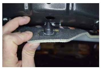
Release the center rear headliner retaining clip using a small screwdriver to release the two tabs on either side of the clip.
