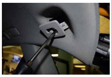
Reinstall the two left and right screen separator mounts and tighten the T-45 Torx screws to 9 Nm.
