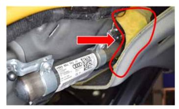
Remove and discard the foam padding from the headliner on the right and left side by gripping the foam padding with the fingers and peel the foam away from the headliner.
