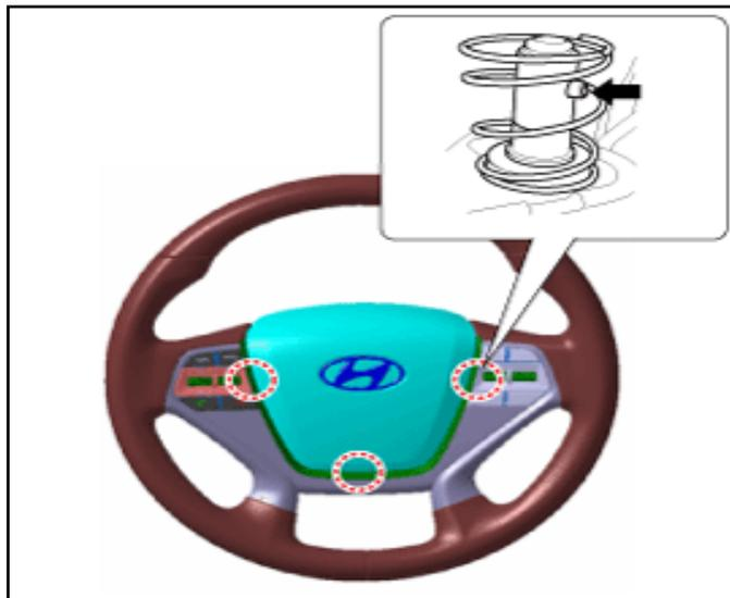
5. Insert a small flathead screwdriver into the locking hole, and press on the 3 snap fit pin stopper to release the Driver Air Bag (DAB) module.
