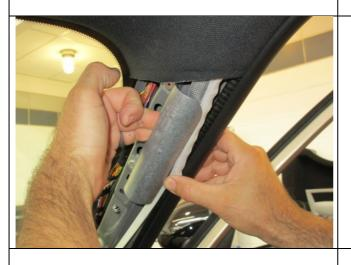
3. Carefully push the air bag package out from behind the metal bracket.
