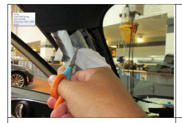
8. Using the round tip scissors, cut off the end of the wrapper at the marked 80mm split line.
