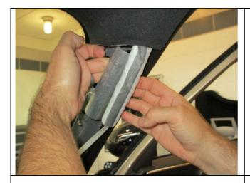
4. Squeeze the air bag package into an oval shape. This will enable it to clear the metal bracket.
