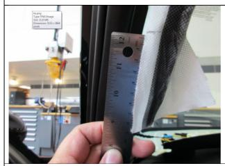
5. Using a metric ruler, mark exactly 80mm up from the bottom of the air bag package.
