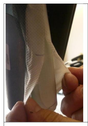
6. Tear open the wrapper, at the split line, from the end of the air bag up to the 80mm mark.
