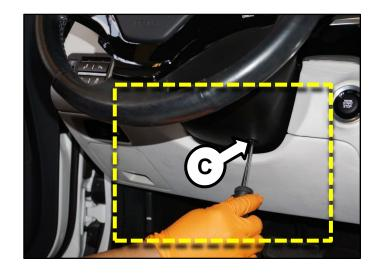
Use a plastic panel remover to separate the upper steering column shroud (D) from the lower section, as shown.
