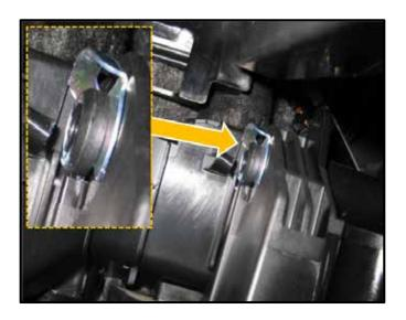
Using a mirror and shop light, inspect for presence of silver-colored locking circlip <arrow> located at the left-hand side of the bearing bracket for the brake pedal and ensure it is fitted correctly on the bearing pin.
