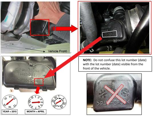
**IMPORTANT:** Only turbocharger air intake ducts with a lot number (date) of **APRIL** (Month 4), 2015 require replacement. If the duct requires replacement based upon the date code, proceed to Replacement Procedure section. If the lot number (date) is confirmed to be **OTHER THAN APRIL**, 2015 (Month 4), the turbocharger air intake duct does **NOT** need to be replaced. Continue on to undercover reinstallation.
