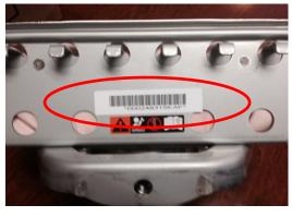
Because this new part is a complete airbag assembly with a different style inflator installed, <u>you do not</u> <u>need to record the old or new inflator</u> <u>serial numbers</u>.
