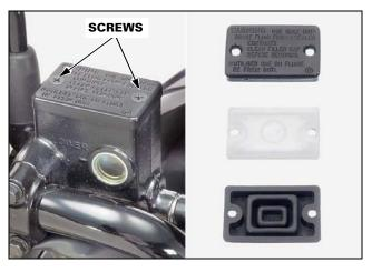
If there is evidence of brake fluid leakage on any plastic or rubber body parts, proceed to DEALER SUPPORT and contact TechLine for further instructions.
