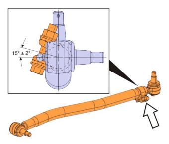
11. Position the replacement draglink rod on the pitman arm as shown in the figure below.
