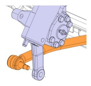
10. Adjust the replacement drag link rod to length for the correct steering wheel angle. Adjust the drag link rod to length and torque the clamp fastener as shown in the figure below.
