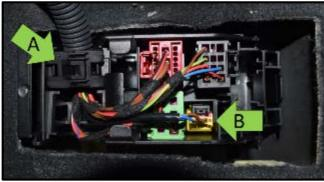
Disconnect the Airbag Lockout Adapter VAS6282 from the side airbag connector <arrow>.
