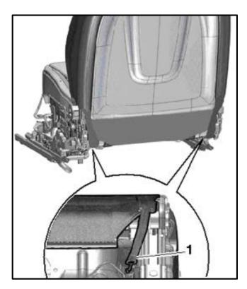
• Detach the rubber strap <1> from the left and right side at the bottom of the seat pan.
