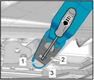
Unclip the cover <1> on the belt relay
