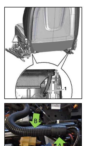
Reattach the rubber straps <1> to the seat pan.
