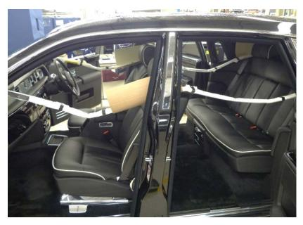
Lower the curtain airbag in preparation for inspection into the position shown.
