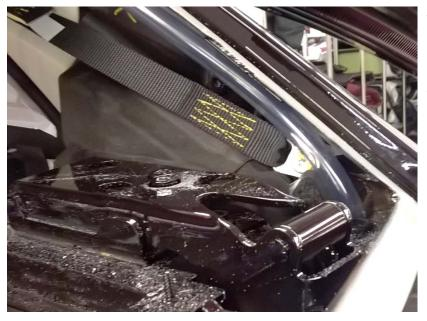
The rear airbag fixing is now accessible once both rear storage shelves are removed.
