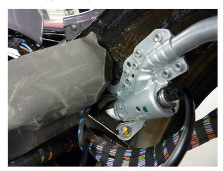
Removing and installing/replacing left curtain airbag ISTA REP 72 12 045 (remaining two fixings)
