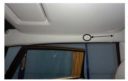
On EWB vehicles the rear roof pillar trim is extended. The front fixing is fragile and extra care must be taken during removal. The fixing is located 330mm from the front of the trim as highlighted.
