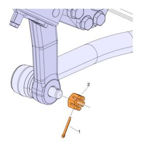
9. Using tool 9996201 (Puller), remove the existing drag link from the pitman arm as shown in the figure below.
