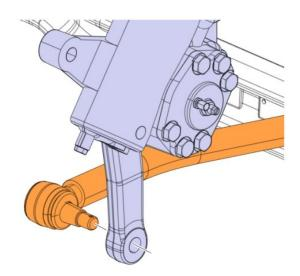
10. Adjust the replacement drag link rod to length for the correct steering wheel angle. Adjust the drag link rod to length and torque the clamp fastener as shown in the figure below.
