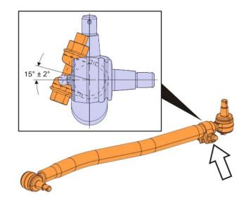
11. Position the replacement draglink rod on the pitman arm as shown in the figure below.
