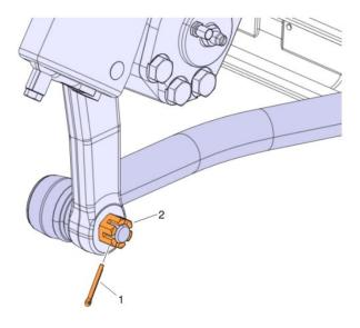
16. Position the replacement drag link rod at the steering knuckle as shown in the figure below.
