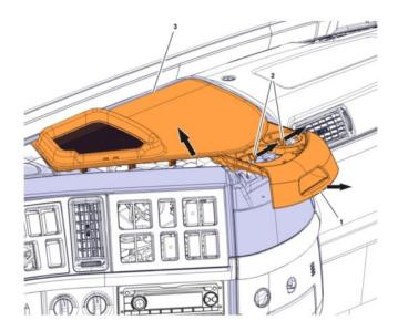
5. Remove the lower dash panel as shown in the figure below.
