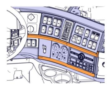
8. Grasp the trailer hand brake trim panel by the top, pull, lift up, and out.
