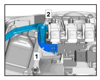
Free up the brake booster vacuum hose <2> on the bracket <1>.
