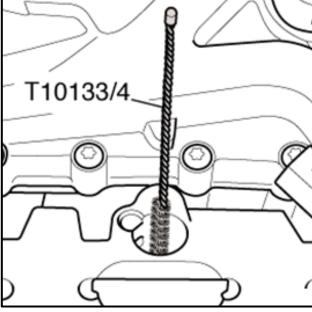
cylinder head with the nylon cylinder brush T10133/4 <as shown>.
