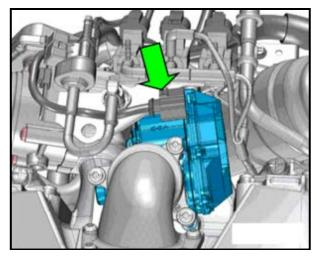
□ Disconnect the control module (J808) <arrow>.
