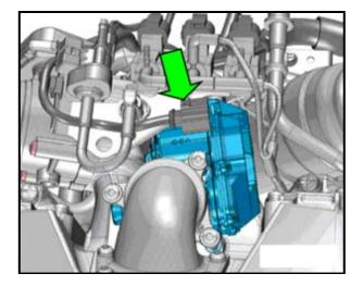
Reconnect the connector <arrow> on the control module J808.
