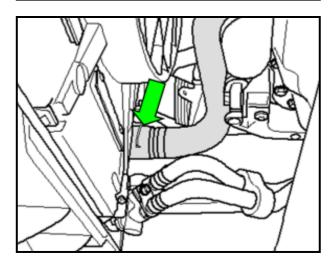
If drain plug is not present and if not already done, reinstall the right lower coolant hose <arrow> onto the radiator, then close the clamp.
