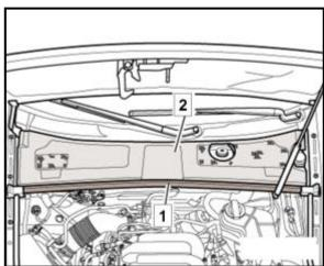
Remove the seal <1> and remove the plenum chamber cover <2>
