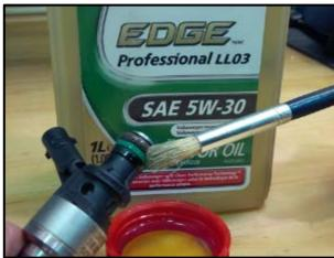
Coat the upper fuel injector O-rings <as shown> with clean engine oil.
