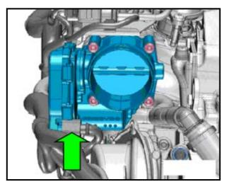
Reconnect the connector <arrow> on the throttle valve control module J338.
