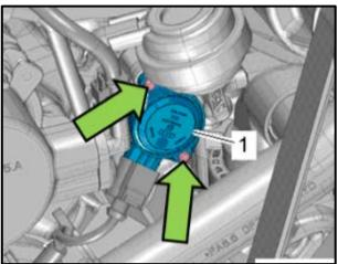
Remove the mounting screws <arrows> from the right Intake Manifold Runner Position Sensor –G336- <1> and position it to the side.
