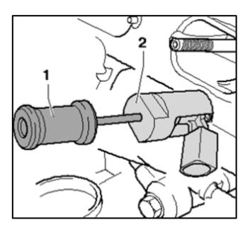
If the fuel injector does not fit into the head by pressing gently, use the puller – T10133B/2A <2> with the Sliding Hammer T10133A/3 <1> to guide the fuel injector into place.
