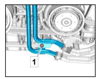
← Remove the coolant hose mounting screw <1>.
