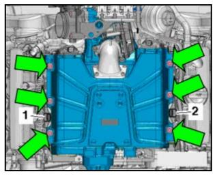
Reinstall the supercharger and torque the nuts <arrows> to 20Nm.
