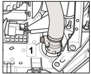
If equipped, open the drain plug <1> and drain the coolant.
