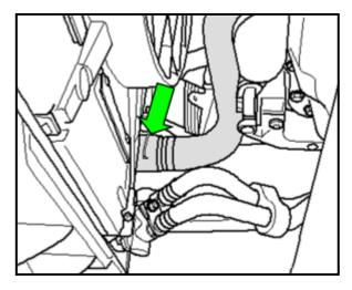
If the drain plug is not present, disconnect the right lower radiator hose <arrow> and allow the coolant to drain.
