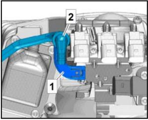
Reinstall brake booster vacuum hose <2> onto the bracket <1>.
