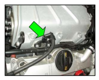
On left side of engine, reconnect electrical connector <arrow> for Charge Air Pressure Sensor 2 G447.
