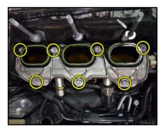
Remove the mounting fasteners <circles> from the intake manifold/fuel rail assembly.
