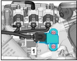
Reconnect the connector on the intake air temperature sensor G42/manifold absolute pressure sensor G71 <1>.
