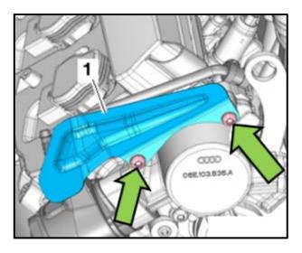
Remove the mounting screws <arrows> and the protective plate <1>.
