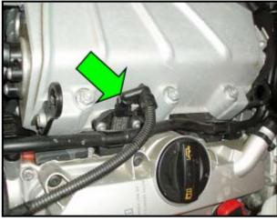
On the left side of the engine, disconnect the Charge Air Pressure Sensor G447 <arrow>.
