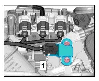
Disconnect the intake air temperature sensor G42/manifold absolute pressure sensor G71
