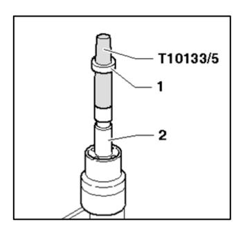
Place the assembly cone T10133/5 with the new combustion chamber seal <1> onto the fuel injector <2>.
