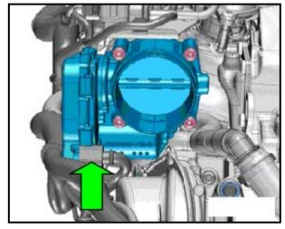
Disconnect the throttle valve control module J338 <arrow>.
