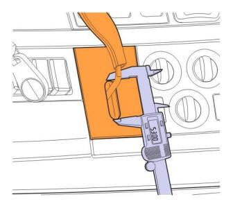
3. If the slot in the trim panel is greater than 59mm, then replacement of the part is not required. Please proceed to commission the vehicle and fill in and return the customer response card. (sample below)
