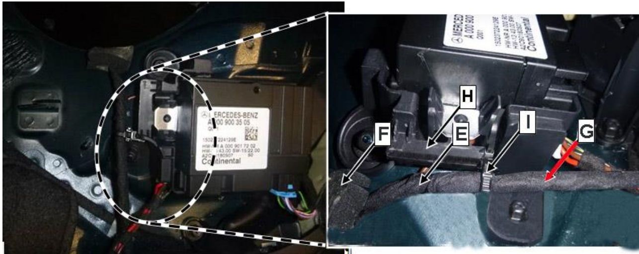
Figure 5 (New wiring harness routing)
