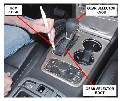
Figure 1 - Gear Selector Boot
