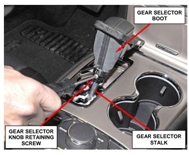
Figure 2 - Gear Selector Knob
