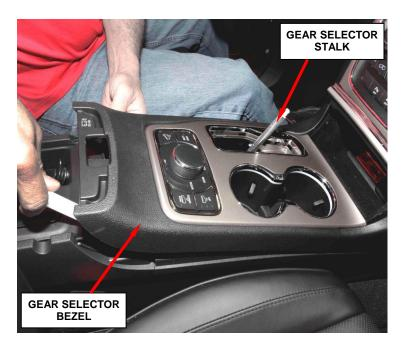
Figure 3 - Gear Selector Bezel
