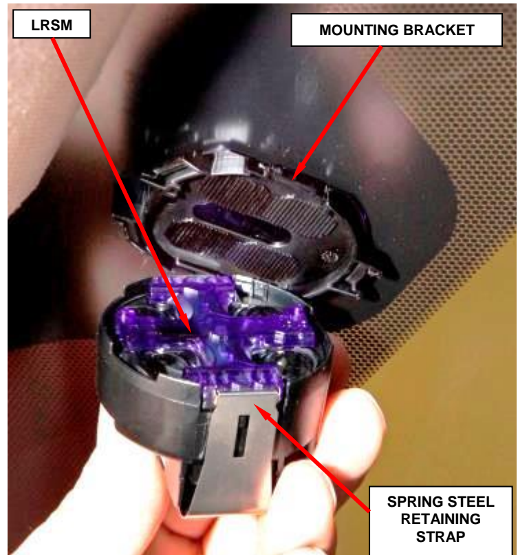
Figure 1 – Light Rain Sensor Module
