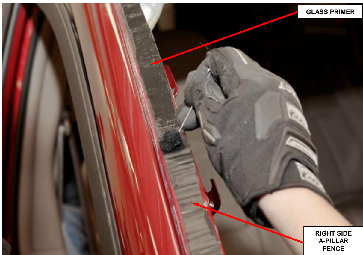
Figure 9 – Windshield Fence Glass Primer
