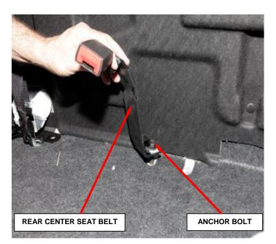
Figure 5 – Seat Belt Anchor
