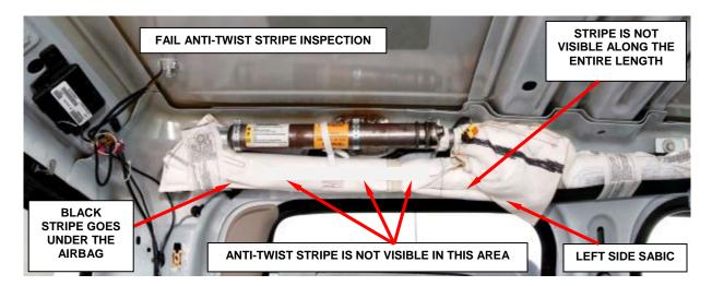
Figure 23 - Failed Inspection: Anti-Twist Stripe Position (Black Stripe for Early Builds)
