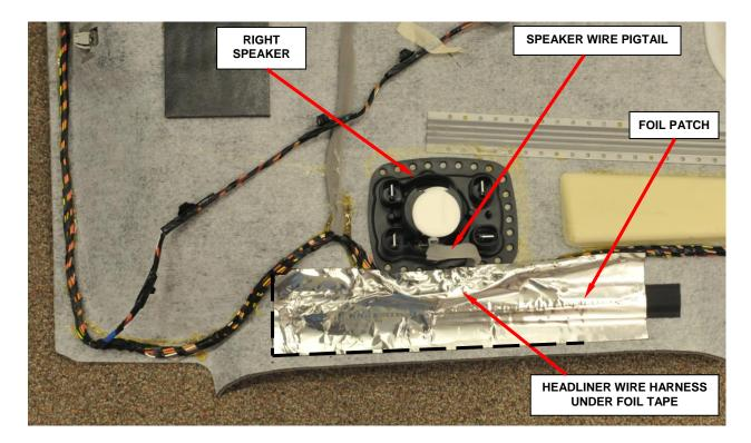
Figure 34 – Foil Patch Installed (Right Side Shown)
