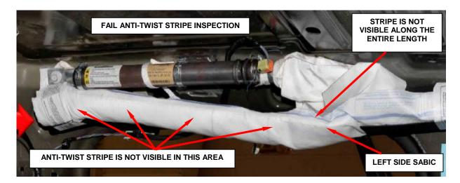
Figure 22 - Failed Inspection: Anti-Twist Stripe Position (Red or Blue Stripe for Late Builds)
