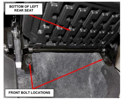
Figure 2 – Left Rear Seat Bolt Locations
