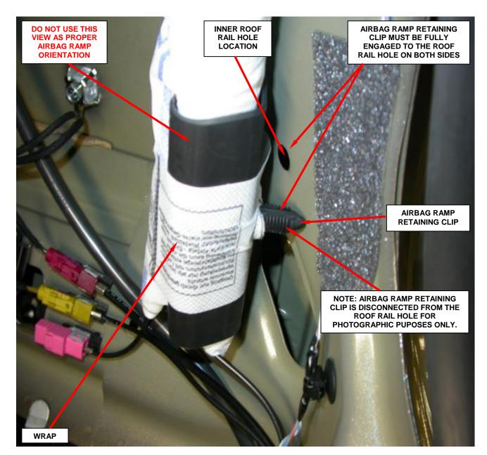
Figure 24 – Airbag Ramp Position (Left Side Shown)
