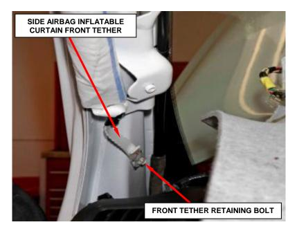
Figure 30 – Tether Retaining Bolt
