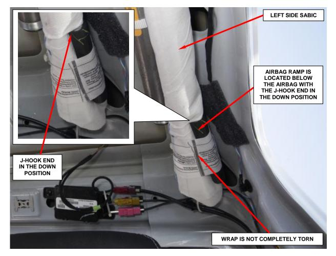
Figure 25 – Passed Inspection: Airbag Ramp and Wrap
