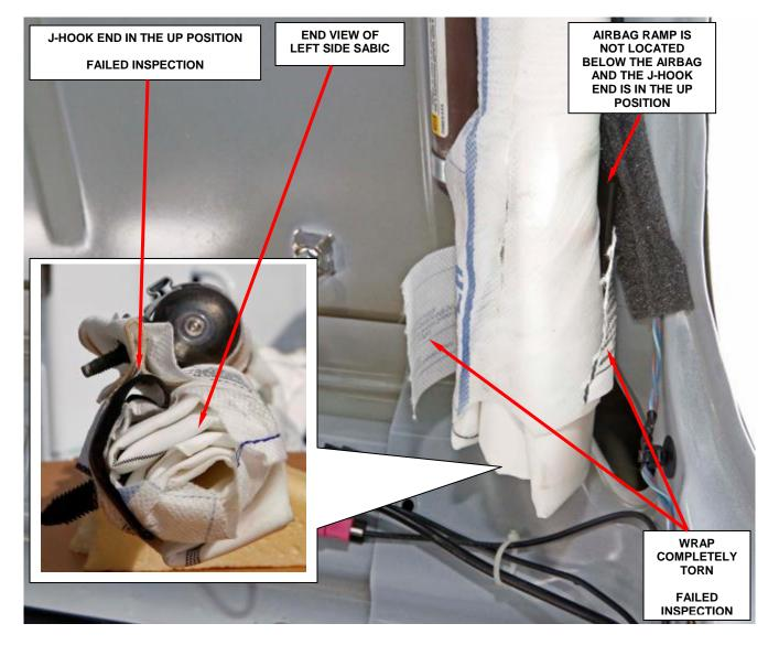
Figure 26 – Failed Inspection: Airbag Ramp and Wrap (Left Side SABIC Shown)
