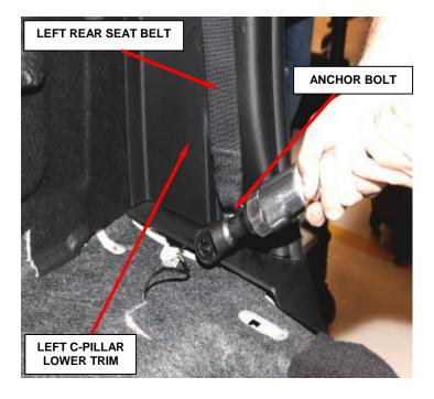
Figure 7 – Left Rear Seat Belt Anchor
