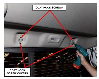
28. Using a small flat bladed tool, open the coat hook screw cover and remove the screws and coat hooks (Figure 17).
