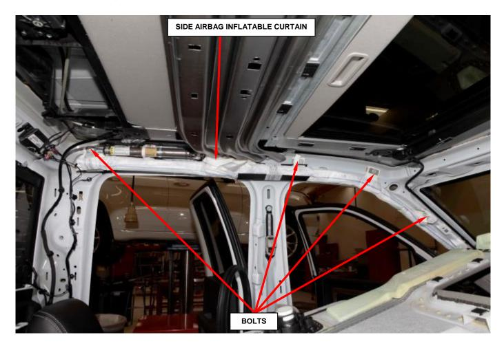
Figure 27 – Side Airbag Inflatable Curtain Bolt Locations
