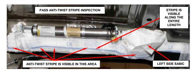
Figure 20 - Passed Inspection: Anti-Twist Stripe Position (Red or Blue Stripe for Late Builds)
