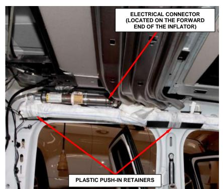
Figure 29 - Plastic Push-in Retainers
