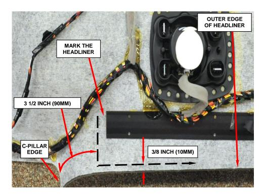
Figure 33 - Mark 3/8 inch (10mm) Location on Headliner
