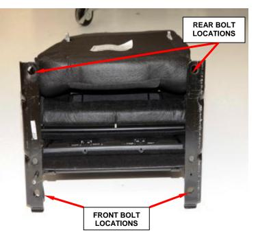
Figure 3 – Left Rear Seat Bolt Locations (Shown out of Vehicle for Photographic Purposes)
