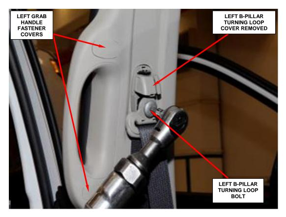
Figure 13 – B-Pillar Turning Loop
