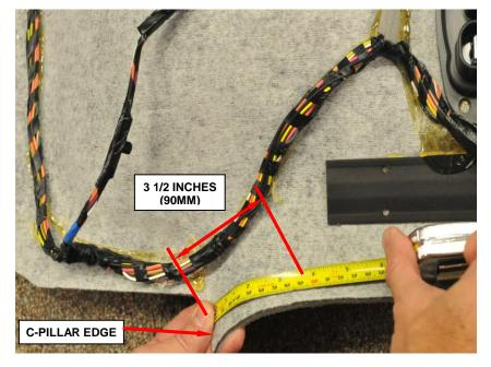
Figure 32 – Mark 3 ½ inches (90mm) Location on Headliner
