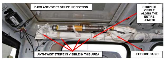
Figure 21 - Passed Inspection: Anti-Twist Stripe Position (Black Stripe for Early Builds)
