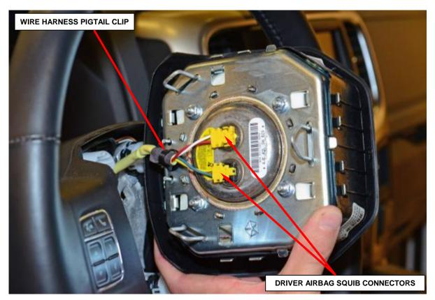
Figure 3 – Driver Airbag Squib Connectors
