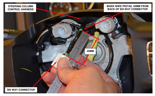
Figure 6 – Mark Wire Harness for Reference
