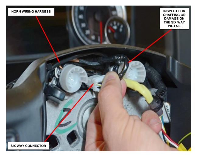
Figure 4 – Inspect For Wire Pigtail Damage
