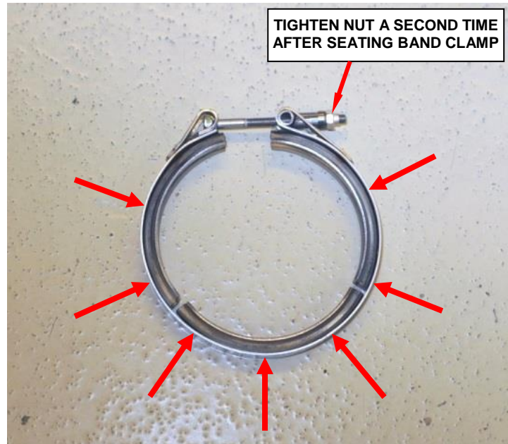
Figure 12 – Tap Around the Clamp with a Hammer to Seat Band Clamp
