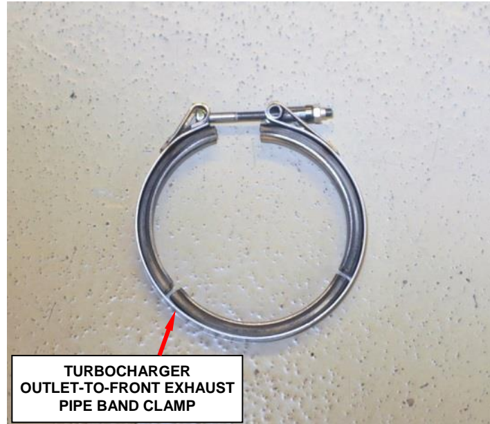
Figure 10 – Turbocharger Outlet-to-Front Exhaust Pipe Band Clamp
