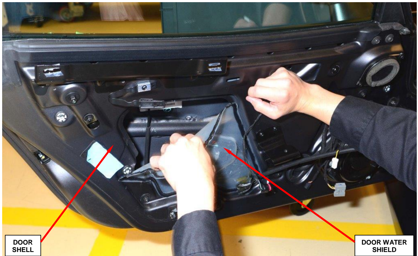
Figure 5 – Partially Remove the Door Shell Water Shield
