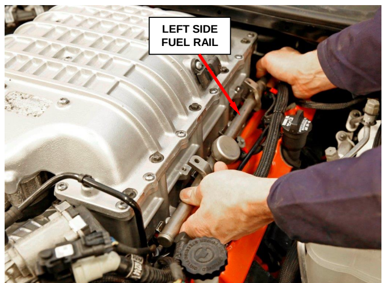
Figure 11 – Rock and Lift Fuel Injector Fuel Rail
