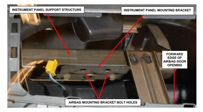
Figure 50 – Instrument Panel Mounting Bracket Viewed through Windshield and Airbag Door Opening
