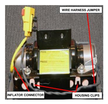
Figure 44 – Wire Harness Jumper
