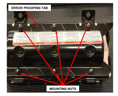
Figure 26 – Mounting Nuts
