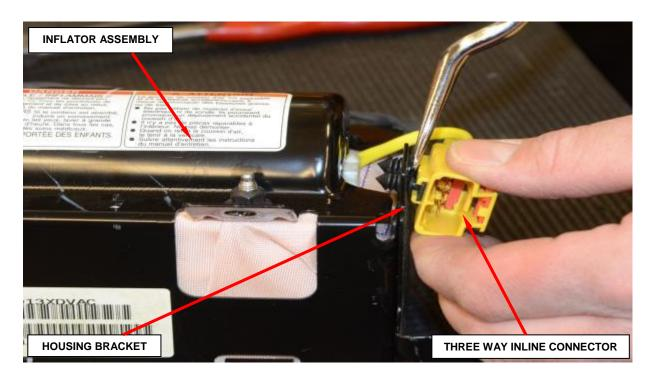
Figure 20 – Yellow Three Way Connector
