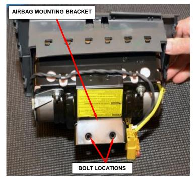
Figure 49 – Passenger Airbag Mounting Bracket e 50).
