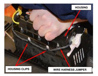
Figure 18 - Wire Harness Clips
