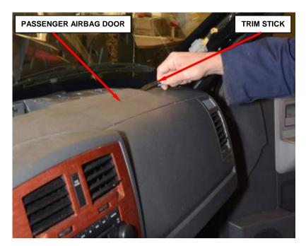
Figure 51 – Passenger Airbag Door
