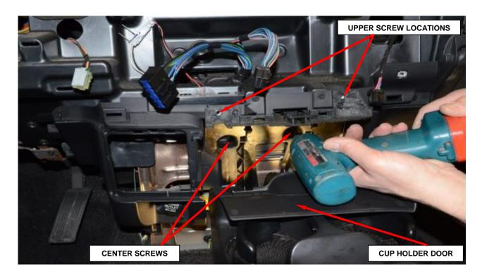
Figure 10 – Center Cup Holder Screws
