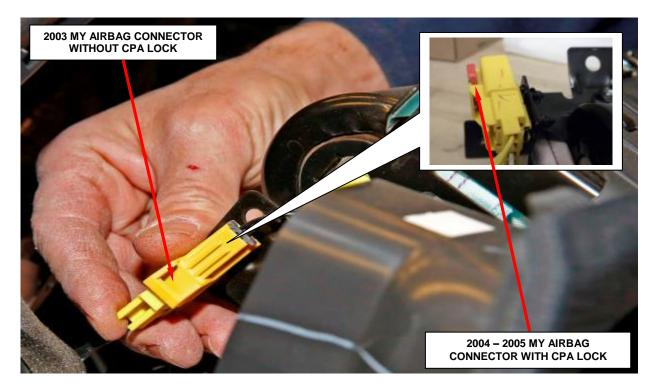
Figure 17 – Passenger Airbag Connector
