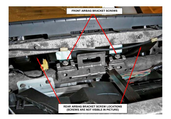
Figure 15 – Passenger Airbag Bracket Screws
