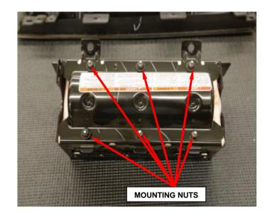
Figure 23 – Six Mounting Nuts
