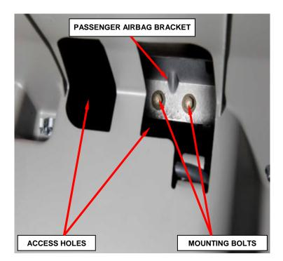
Figure 30 – Airbag Mounting Screws and Bracket
