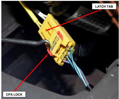
Figure 33 – Airbag Inflator Pigtail Connector
