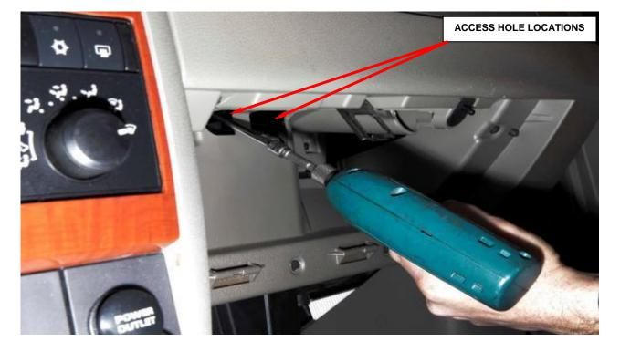
Figure 31 - Passenger Airbag Mounting Bolt Access Holes
