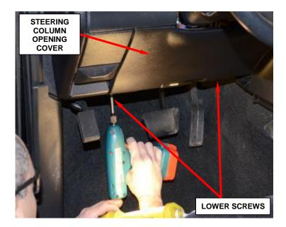
Figure 4 – Steering Column Opening Cover
