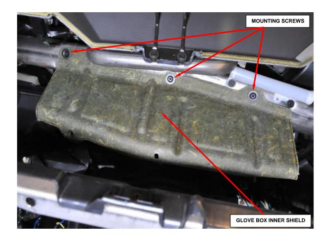
Figure 41 – Inner Glove Box Shield
