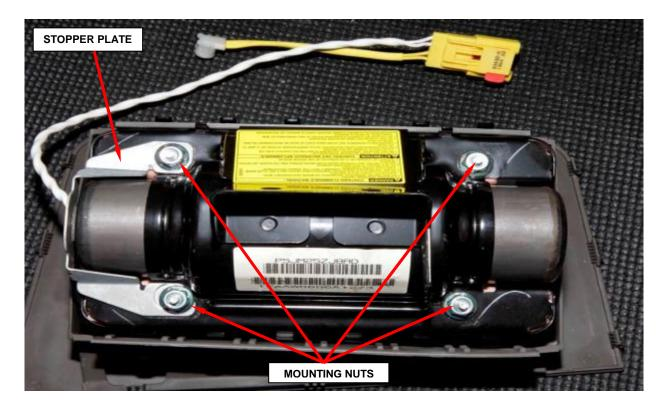
Figure 55 – Mounting Nuts and Stopper Plate
