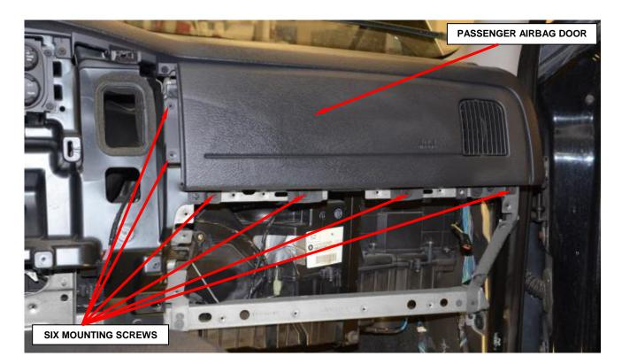
Figure 14 – Passenger Airbag Door Mounting Screws
