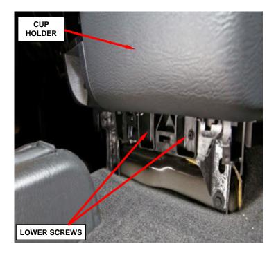
Figure 9 – Lower Cup Holder Screws
