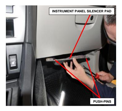
Figure 39 – Instrument Panel Silencer
