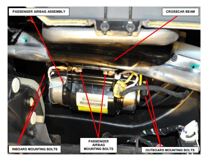
Figure 42 – Passenger Airbag Mounting Locations
