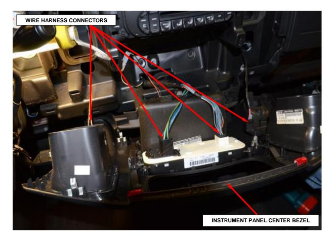
Figure 6 – Center Bezel Wire Harness Connectors
