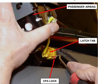
Figure 52 – Airbag Inflator Pigtail Connector
