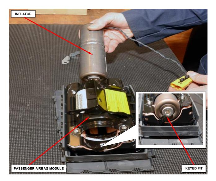
Figure 57 – Passenger Inflator Installation
