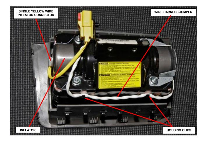
Figure 34 – Passenger Airbag Assembly
