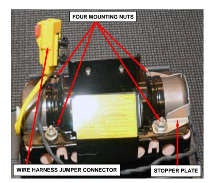
Figure 45 – Airbag Module
