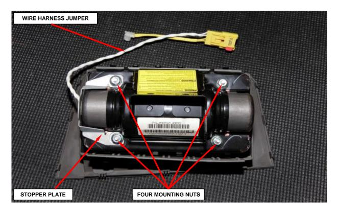
Figure 36 – Mounting Nuts and Stopper Plate
