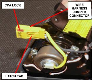
Figure 43 – Wire Harness Jumper
