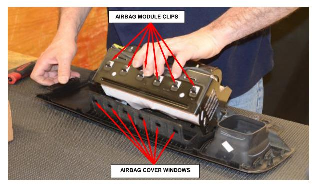
Figure 22 – Airbag Cover Clips
