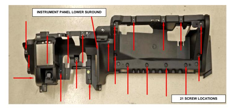
Figure 12 - Instrument Panel Lower Surround Screw Locations
