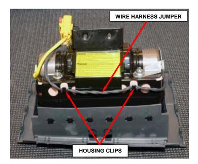
Figure 53 – Passenger Airbag Assembly
