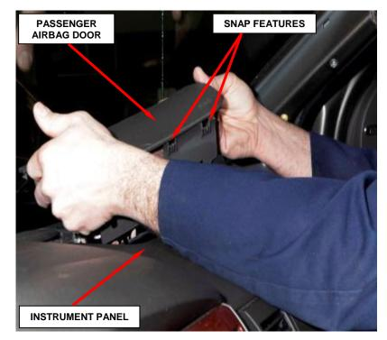
5. Pull the passenger airbag out of the instrument
