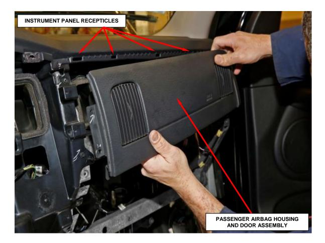
Figure 16 – Passenger Airbag Housing and Door Unit
