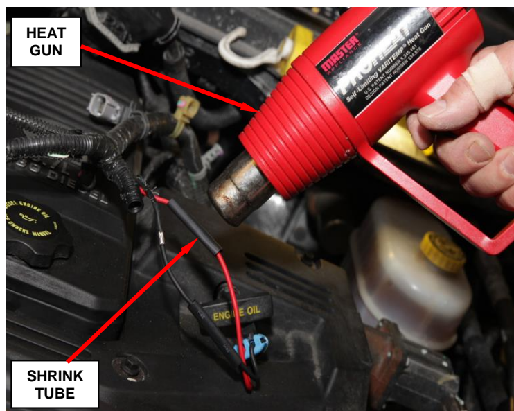
Figure 16 – Install Heat Shrink Tube
