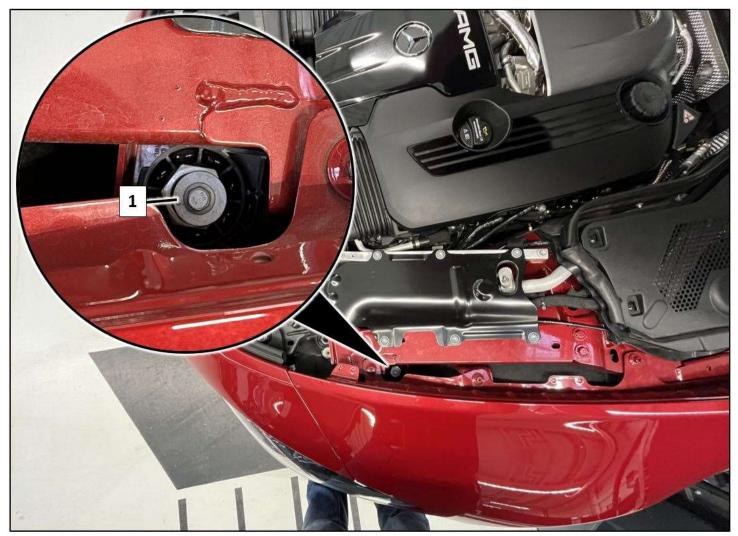
Figure 1: Washer on left headlamp shown
