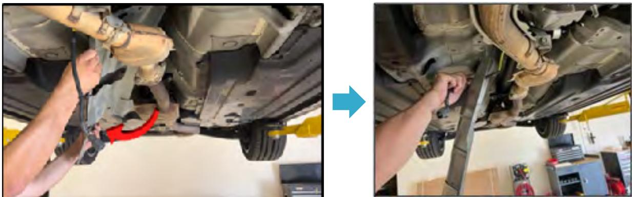
**STEP 15:** Remove the snap pin and washer from the reverse check cable. These parts will be reused and should be stored securely. Once removed, disconnect the cable from the reverse check lever.
