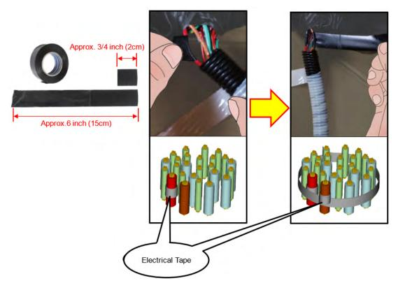
**STEP 13:** Wrap the repaired area using the original white tape around the corrugated tubing. If needed, use a piece of electrical tape to secure the end of the white tape. Proceed to Step 15 when complete.
