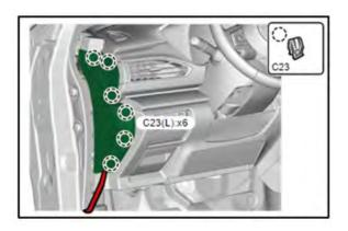
**STEP 3:** Pull the front left side cover in the horizontal direction to release the holding claws. Once released remove the cover.
