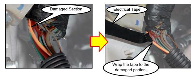
STEP 12: Wrap the remaining tape around the entire wiring harness.
