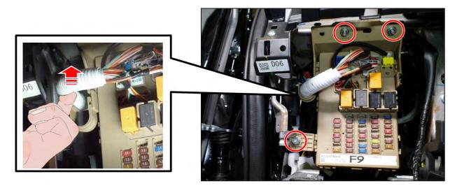
**STEP 6:** Position the fuse panel toward the floor of the vehicle. This will allow the required workspace needed for the following Steps.
