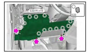
**STEP 5:** Release the instrument panel harness from the mounting hook located on the side of the fuse panel. Release the two mounting nuts and one mounting bolt.
