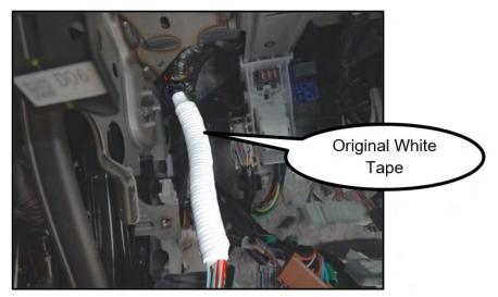
**STEP 14:** Remove the instrument panel assembly as per the applicable Service Manual and replace the instrument panel harness. Refer to STIS: <u>Body & Electrical/WIRING SYSTEM ></u> <u>Instrument Panel Assembly</u>
