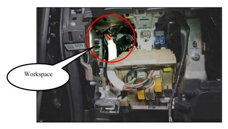
**STEP 7:** Push the instrument panel harness downward by hand. CAREFULLY inspect the wires close to the edge of the steering beam bracket as shown in the picture below.
