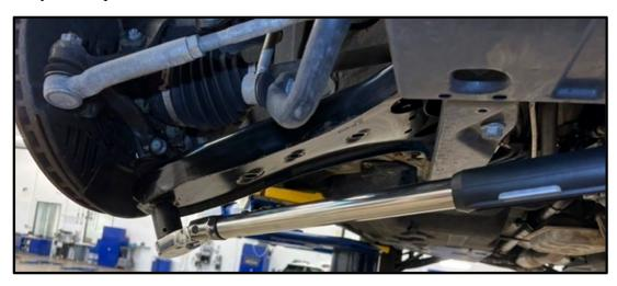
**STEP 6:** Perform a visual inspection of the markings made to the castle nut and lower control arm. If the markings indicate the castle nut has moved during the torque procedure, the lower control arm assembly will require replacement. If the markings indicate no movement, only the cotter pin will require replacement. See the images below.
