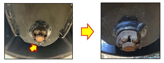
**STEP 4:** Using a paint marker, mark an alignment line on the joint portion of the lower control arm and the castle nut. See the images below.
