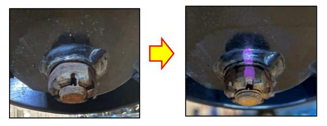
**STEP 5:** Set a torque wrench to 39Nm (28.8ft. lbs.). Tighten the castle nut until the torque limit is indicated by the torque wrench.
