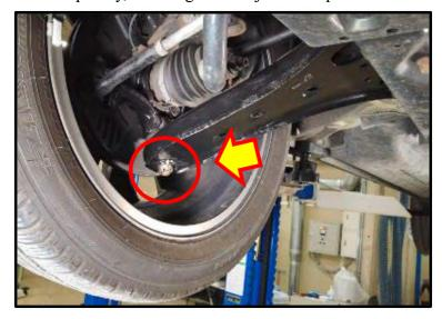
If the ball joint separates from the lower control arm while driving, the vehicle may experience a loss of control, increasing the risk of a crash.
