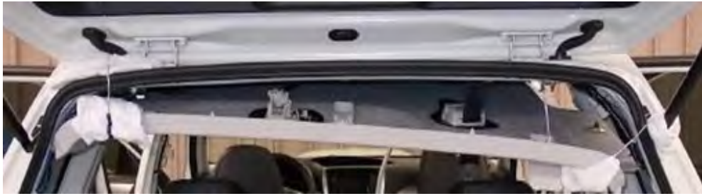
Headliner supports in place
