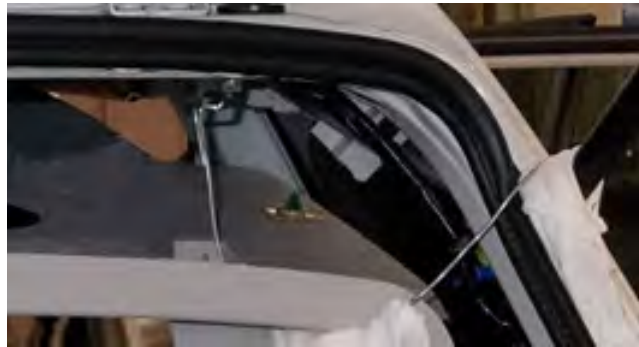
Right side headliner support Hook to tether anchor, then route through headliner opening for tether and attach to rear gate stay.
