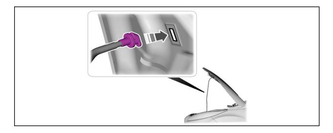
**STEP 6** Locate the existing VECI label on the inside of the hood, as shown in the image below.
