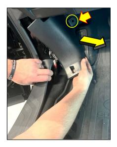
**CAUTION:** ALWAYS remove the cover when it is or has reached room temperature. Any attempts of removal in cold ambient temperatures may result in unwanted breakage. DO NOT use excessive force when pulling the covers. This may cause damage to the covers.
