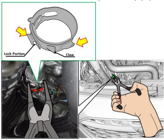
**STEP 5**: Using 35-45° bent long-neck needle nose pliers, squeeze the lock portion of the clamp, and confirm it is fully locked.
