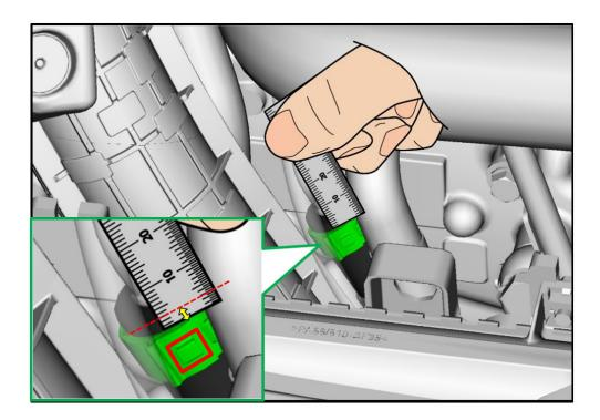
**STEP 4:** Using 35-45° bent long-neck needle nose pliers, squeeze the clamp at the two points indicated with arrows below. Confirm the lock portion is hooked properly onto the claw.
