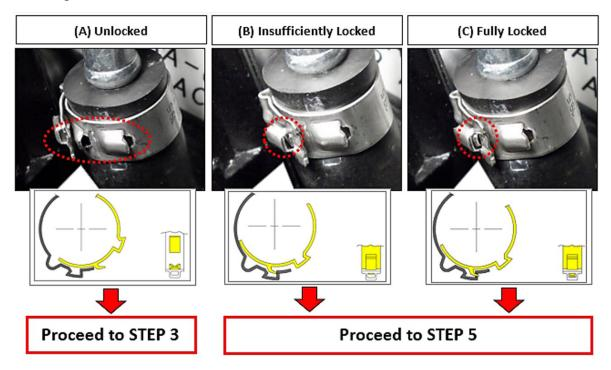
**STEP 3:** Adjusting the hose clamp position.
