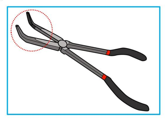
**NOTE:** The Snap On® 11" Talon Grip™ Long-Neck 35° Bent Needle Nose Pliers (#411CF) are a usable suggestion.
