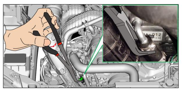
**STEP 6:** Confirm the clamp is fully locked by visually inspecting the claw position as shown in the image below.
