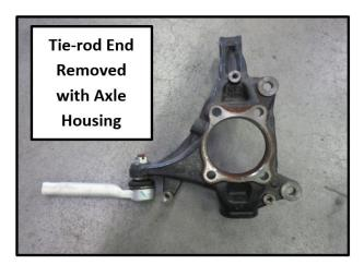
**IMPORTANT NOTE: ALWAYS** use new wheel bearing mounting flange bolts, strut self-locking nuts, axle nuts, and tie rod end nuts during assembly. Be sure to torque these items to the correct specification.
