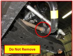
**Tip 2:** Even with usage of a recommended ball joint separator tool (shown below), there can be difficulty separating the tie rod end from the axle housing. This is caused by possible deformation of housing/tie rod from exceeded torque limits during installation. **ALWAYS** use eye protection when attempting to apply this method. If there is difficulty found when removing/separating the tie rod end with the axle housing, follow the procedures outlined on the next page.
