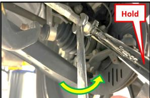
STEP 3: While holding the steering gear box boot (C) and CAREFULLY preventing it from turning, loosen the tie rod (D) with a 14mm wrench. Take note of the number of rotations during removal and apply the rotation number to the new part installation. This will help save time during the alignment. Use CAUTION when performing this STEP to ensure the steering gear box boot does not twist/and or rotate.
