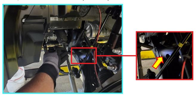
STEP 3): Clean the top of the front lower control arm with a damp cloth to provide increased visibility of the stamped Lot Number. Verify and record the LOT Number with a photograph and document the LOT number on the repair order. A photograph can be taken with the wheel in the left full lock position.
