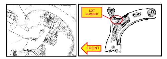
**STEP 3):** Illuminate the stamped LOT Number on the left front lower control arm. Capture the 5 digit Lot Number with a photograph and document the LOT number on the repair order.
